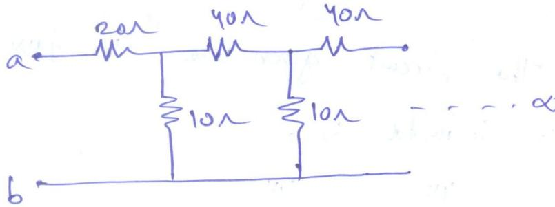
6. for what value of 'a' maximum power transferred to  $20\Omega$  and also maximum value of power in watts respectively.
