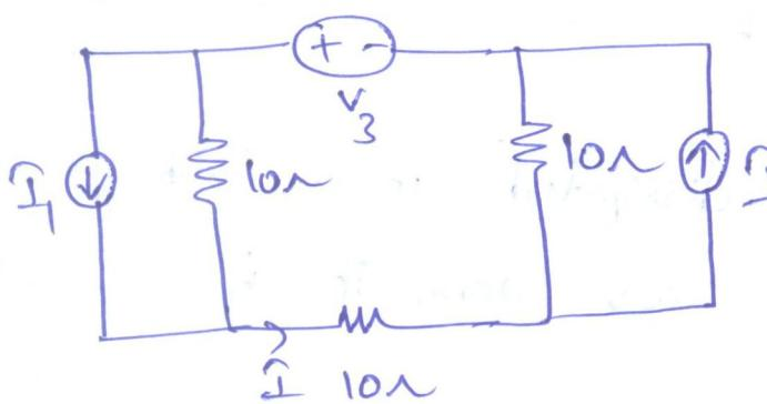
8. In the circuit, if  $I = 2A$ , then the value of the battery voltage  $V$  will be \_\_\_\_ volt.
